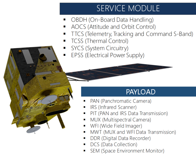
Figure 1. Conceptual View of CBERS–4. [CBERS 2017].
